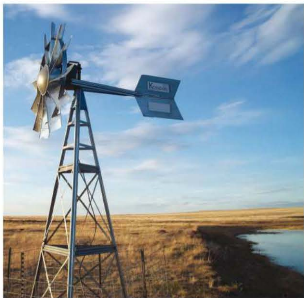
Water-pumping windmills perform on towers only 12 to 25 feet tall (left). Drop-in-stream pumps require minimal upfront installation (right).
