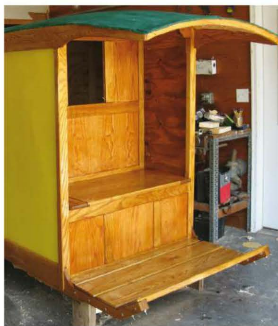
The horse-drawn wagon's cargo area bests the author's station wagon in food-hauling capacity (top). The bench seat on the front holds a car battery to power rear flashers and a dome light, with storage room to spare (bottom).
